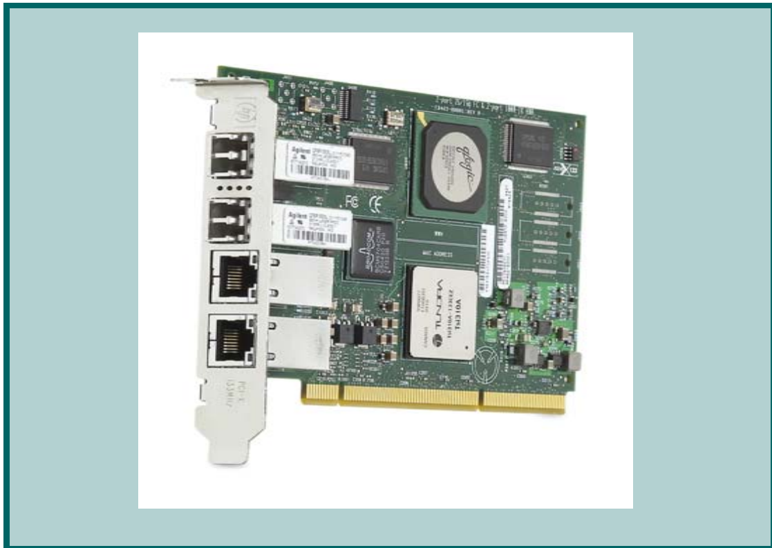
Figure 1 AB465A Combination 2-Port 2-Gbps Fibre Channel / 2-Port Gigabit Ethernet Card
